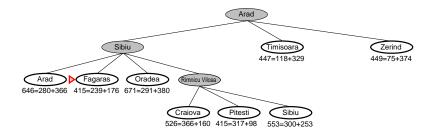
Expand the node Pitesti, because it has the smallest f-value
