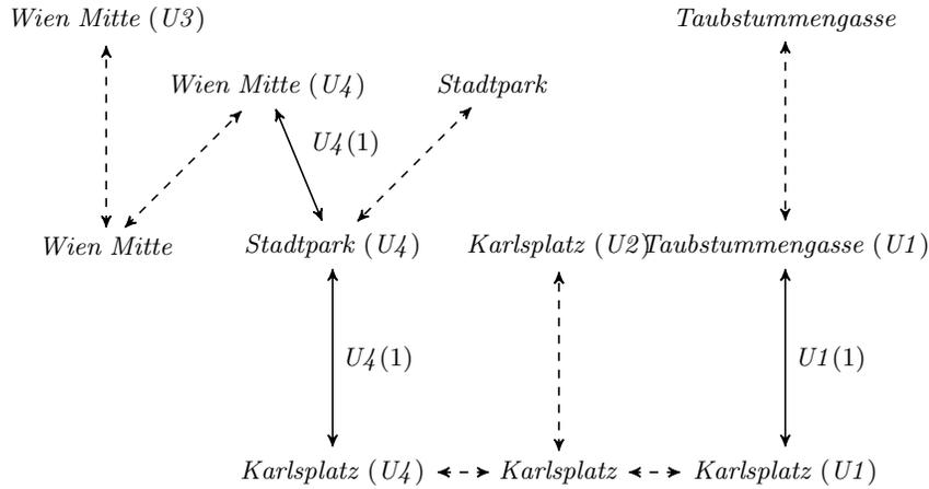
Abbildung 3: Graph representation of stations and lines (dashed: changes with costs 10, solid: given lines and costs)
