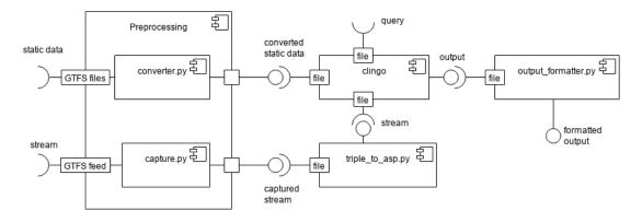
Figure 21: Component diagram for GTFS and clingo
