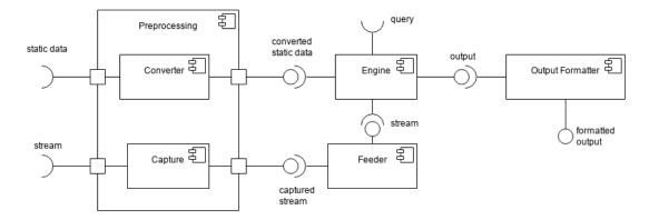
Figure 5: Component diagram of modules
