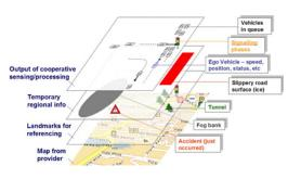
Fig. 1. The four layers of a LDM [2]
